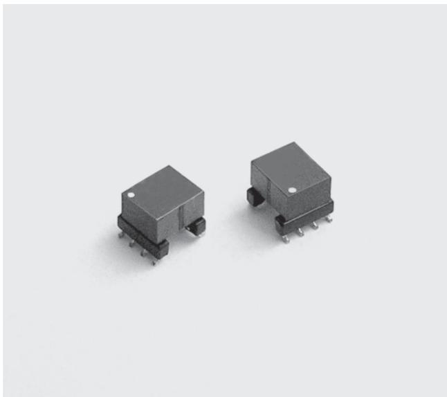
The FA2659-AL gate drive transformer is designed for high switching speed, transformer coupled MOSFET and IGBT gate drive circuits operating from 50 kHz to as high as 2 MHz. It offers low leakage inductance, excellent interwinding capacitance and 2250 Vdc primary to secondary isolation. The miniature surface mount package requires only 56 mm<sup>2</sup> of board space, allowing for high density mounting.
