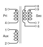
Secondary windings to be connected in parallel on the PC board
